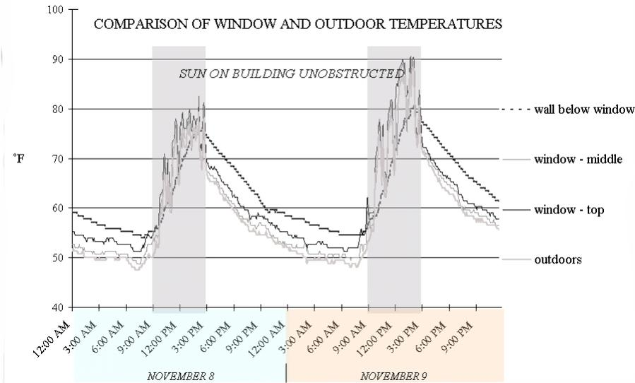
Fig. 13: Comparison of window and outdoor temperatures
