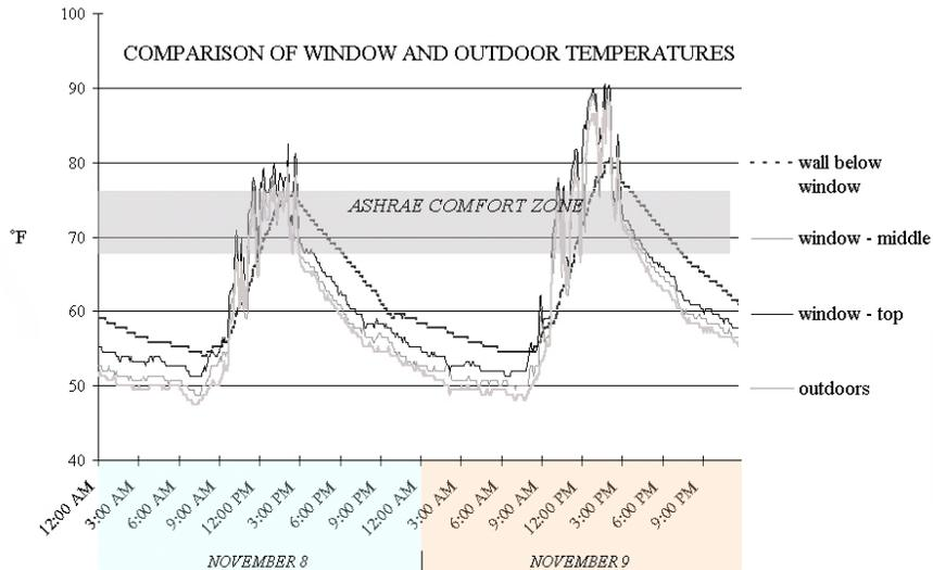
Fig. 7: Comparison of window and outdoor temperatures
