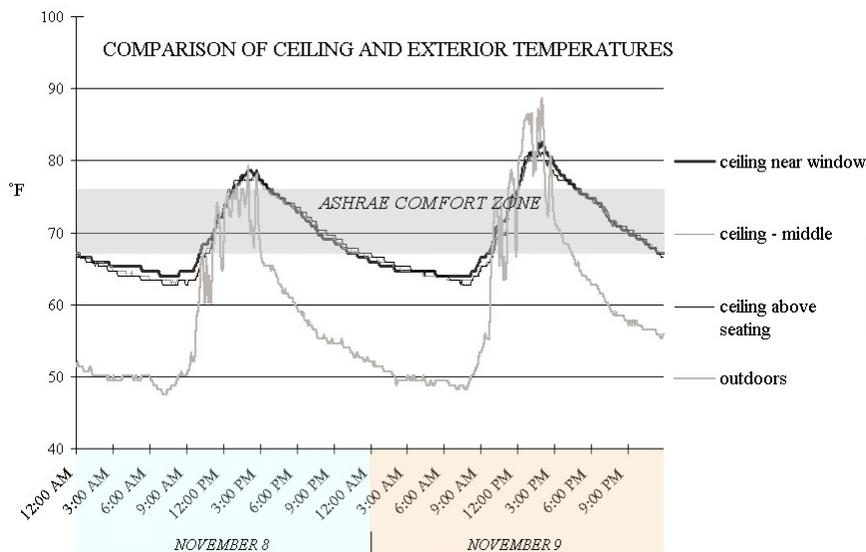
Fig. 8: Comparison of ceiling and outdoor temperatures
