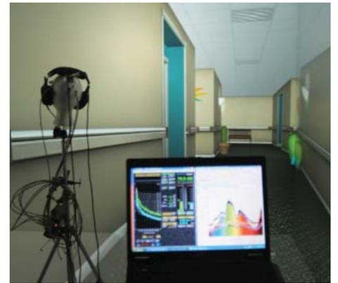
Mr. Manikin Head is measuring spectral characteristics of the surfaces within the VR environment.
