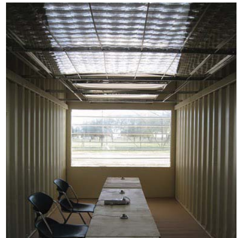
The Horizontal Hybrid Solar Light Pipe forms the ceiling of the unilaterally daylighted test cell.
